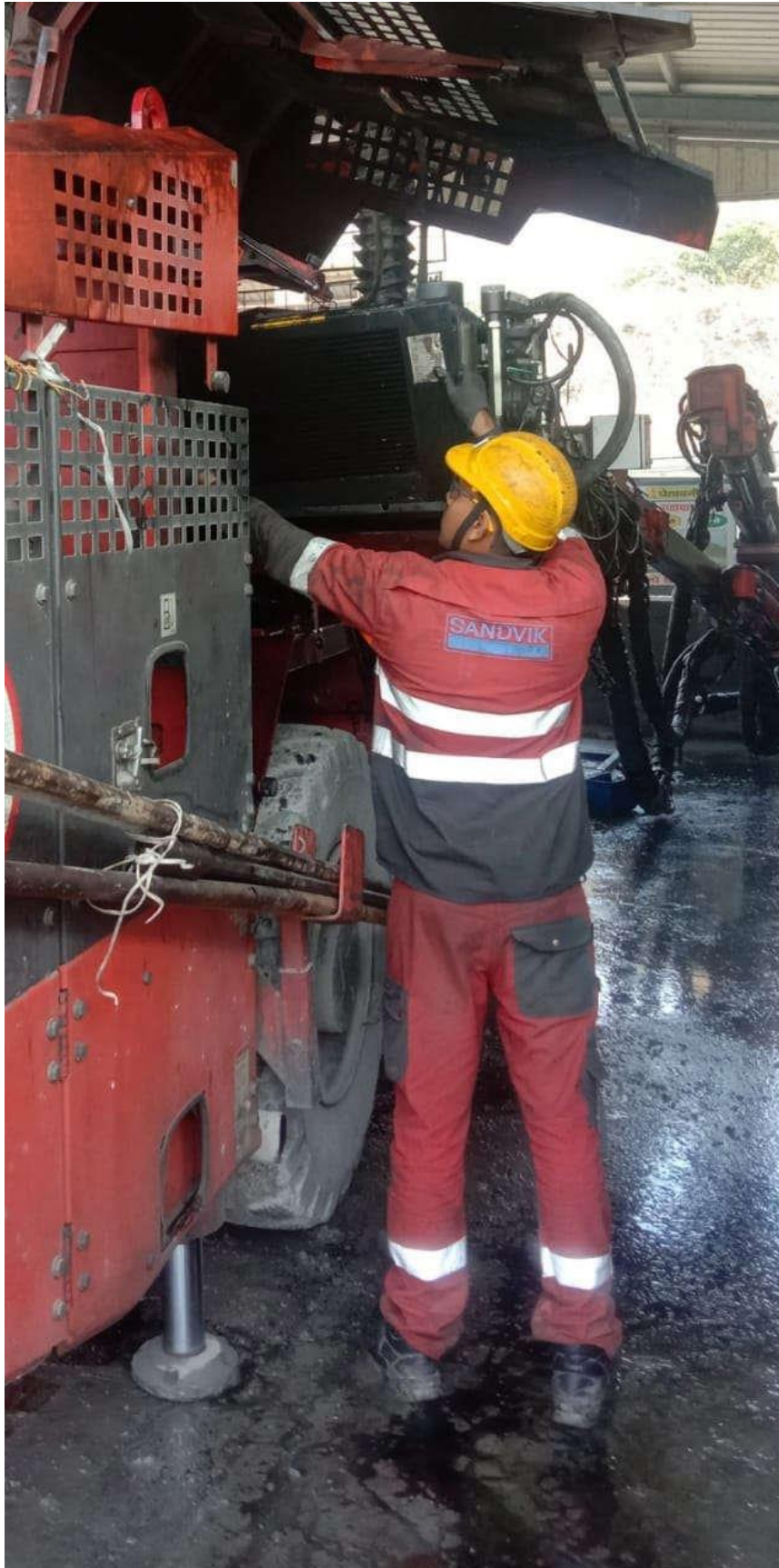
DD321 COMPRESSOR COOLER REPLACEMENT
