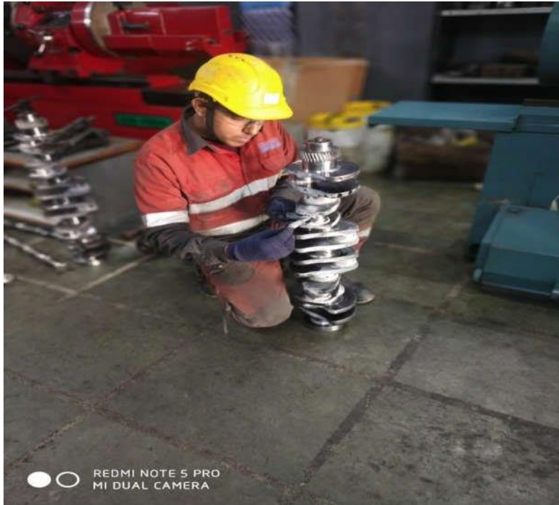
CRANKSHAFT PIN MEASUREMENT HELP OF MICROMETER
